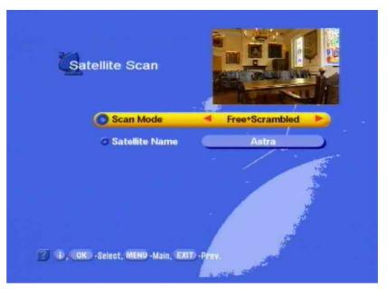
In the "Satellite Scan" menu you set the receiver searching for programmes on a satellite. Move to the menu line you want using the
